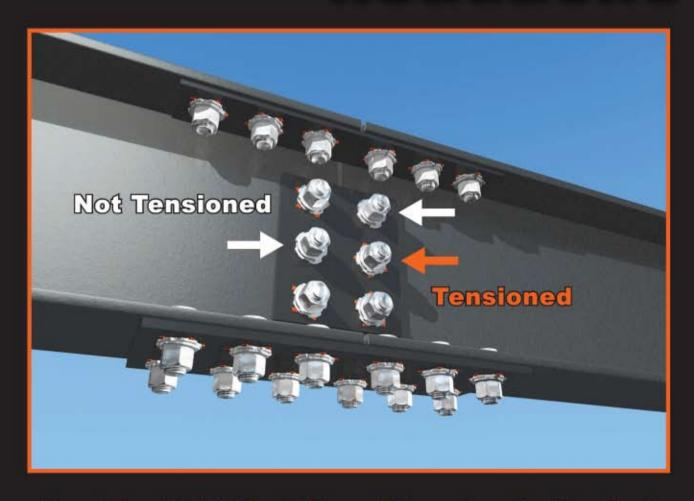
Squirter™ DTI's (Direct Tension Indicator) take the headache out of bolting.
