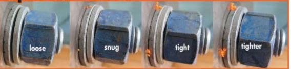
SQUIRTER™ DTI's (Direct Tension Indicator) are DTI's with a flexible silicone embedded in the depressions under the bumps. To use them, simply ... Tighten the bolt until the calibrated amount of orange silicone appears from under the DTI's squirt locations, then stop tightening. That's all there is to it.
