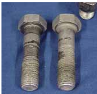
Substantial wear on the threads indicates movement due to incorrect preload.
