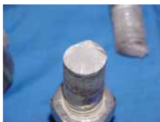
Failure point. Note wear on bolt shank.
